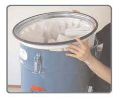
Lift the filter and the holding ring.
