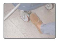
Set on the wheel's brake to ensure that the machine position is stable.
