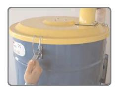
Release the vacuum's head spring hook fasteners.
