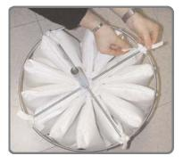
Untie the knots and withdraw the multi-ply filter, reassemble the filter proceeding with care and finally fasten the cover.
