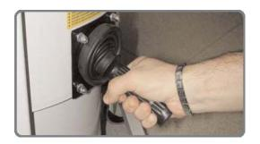
If the optional automatic filter shake system is available, press the blue led switch and keep it pressed for a few seconds to start filter shake functions.
