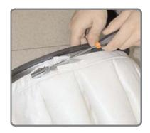
Loosen the clamp and remove the holding ring with the sheath.
