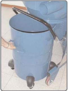
Empty the collection container transferring the collected debris into a specially provided container for waste disposal, complying with the applicable laws and regulations in force.
