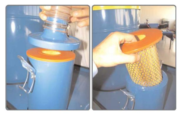
Use another vacuum to clean the cartridge-filter and remove the dust thereon. For assembly, once the cartridge-filter cleaning has been completed, execute the same disassembly operations in reverse order.
