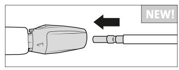
New: Pistol (left) with plug coupling, lances and other Accessories (right) with plug nipple.
