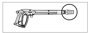
Safety trigger gun (M2000, with extencion) with plug coupling
