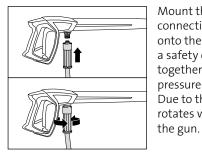
Mount the grey rotating screw connection of the high-pressure hose onto the trigger gun incorporating a safety catch. Afterwards screw together ensuring a snug and pressure-tight fit.
