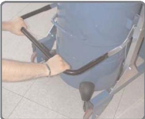
The collection container's fitting and securing operation must be executed by one person only, pushing the shackle down with both hands.
