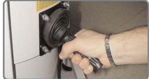
If the optional automatic filter shake system is available, press the blue led switch and keep it pressed for a few seconds to start filter shake functions.
