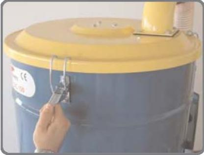
Release the vacuum's head spring hook fasteners.
