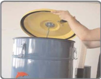
Lift the cover and lay it on the supporting bench.
