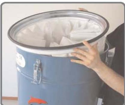
Lift the filter and the holding ring.
