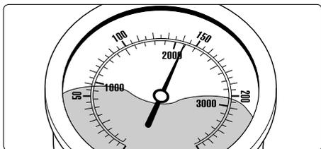
■ **No water from the nozzle but the gauge shows full pressure: Most likely the nozzle is blocked.** (Inside the pressure gauge there is no water but a filling with glycol to damp the vibration of the pointer.)
