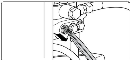
Take a wire (paper clip) and clean valves under running water. Also clean valve seating inside the pump.
