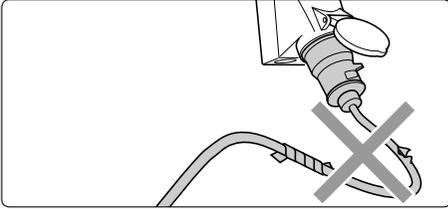
**Only use power cables which are in perfect working order! Do not damage the power cable or repair it incorrectly!**
