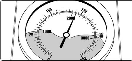
■ The pressure gauge shows full pressure although the gun has been closed. The pressure switch valve switches constantly.
