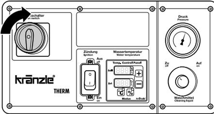
2. Switch on main switch with disengaged spray gun. Vent high-pressure cleaner: Pull and release trigger of spray gun various times.
