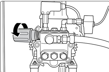
The pressure control valve on the pump head is used to control the operating pressure plus the water flow and consequently the water temperature as well. Turn right to increase the pressure, turn left to reduce the pressure.
