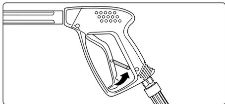
Apply the safety catch on the spray gun after each use, in order to prevent unintentional spraying!
