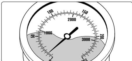
■ **Pressure gauge shows little pressure, the water from the nozzle comes in squirts. The high-pressure hose vibrates. Most likely the valves are soiled.**
