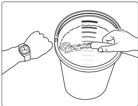
Lack of water occurs more often than you probably believe. The more powerful a high-pressure cleaner is the greater is the danger that a lack of water occurs. If there is only an insufficient amount of water available, cavitation arises inside the pump, which is normally noticed too late or even not at all. The pump will be destroyed. Please check the available quantity of water by filling a bucket with litre scale for one minute.
