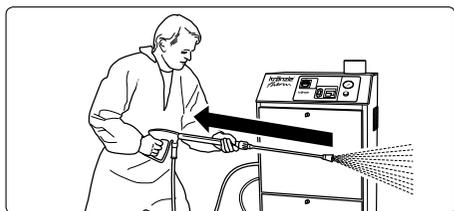
Bear in mind that during cleaning tasks with a high-pressure water jet a significant recoil at the lance arises. Additionally angled lances produce a clearly perceivable amount of torque.
