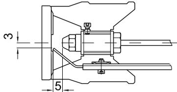
For a smooth ignition, the setting of the ignition electrode must be controlled regularly (after 500 operating hours at the latest).
