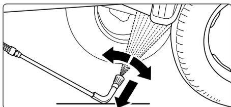
Always aim the underbody lance! Bear in mind when using a curved or angled spraying lance that there is a significant amount of torque in the recoil!
