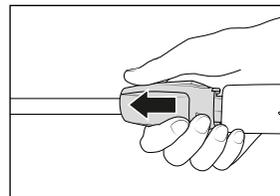
After insertion of the lance, release retaining sleeve and make sure that the lance is in a secure position.
