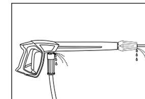
**Proceeding:** Check connections from the high-pressure cleaner to the high-pressure hose and from the high-pressure hose to the safety trigger gun and also the connection between lance and safety trigger gun for tightness.
