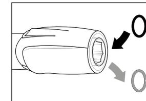
Switch off the cleaner. Shortly press the trigger of the trigger gun with safety catch to decrease the pressure. Remove high-pressure hose, trigger gun with safety catch and lance and check the O-rings. If the O-rings are damaged they have to be replaced.
