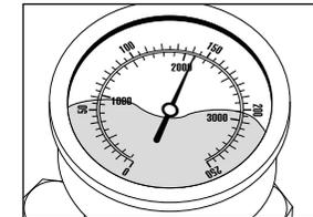
Having closed the trigger gun with safety catch, the high-pressure cleaner must shut down and the stainless steel pressure gauge must show „0“ bar. If not shut down and the stainless steel pressure gauge continuously shows full pressure, this could be due to leakage at the high-pressure pump, at the pressure switch, at the high-pressure hose or at the trigger gun with safety catch.
