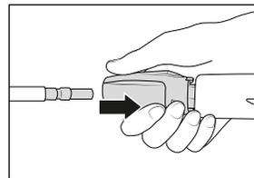
First pull back the retaining sleeve of the safety trigger gun, then insert lance into the plug coupling connection of the safety trigger gun.
