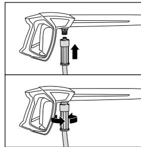
Mount the grey rotating screw connection of the high-pressure hose onto the trigger gun incorporating a safety catch. Afterwards screw together ensuring a snug and pressure-tight fit.
